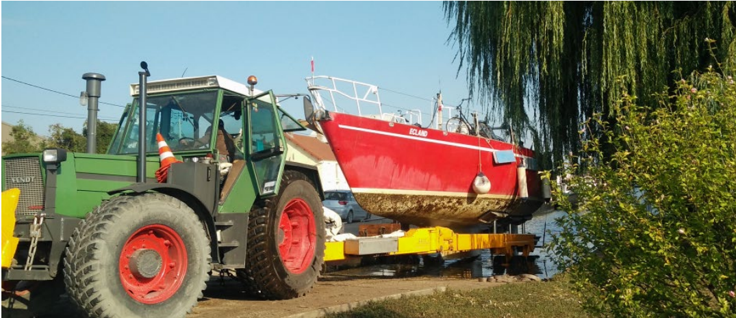
Ecland pulled out from the slip in Saint-Jean-de-Losne. The hull is not very dirty, but it's however worth a sweep with high-pressure water, especially on propeller and tiller.
